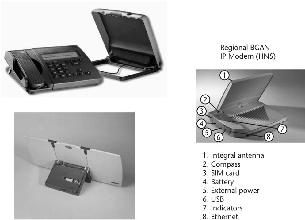
**Figure 11.9** A selection of user terminals for use on the Inmarsat system.
