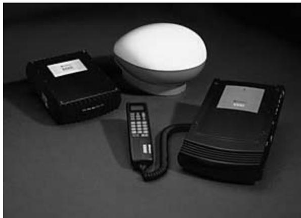
**Figure 11.11** Typical MSAT mobile UTs.
