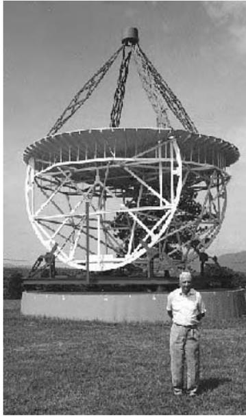
**Figure 1.3** Grote Reber's home-built backyard radio telescope (photo courtesy of NRAO).
