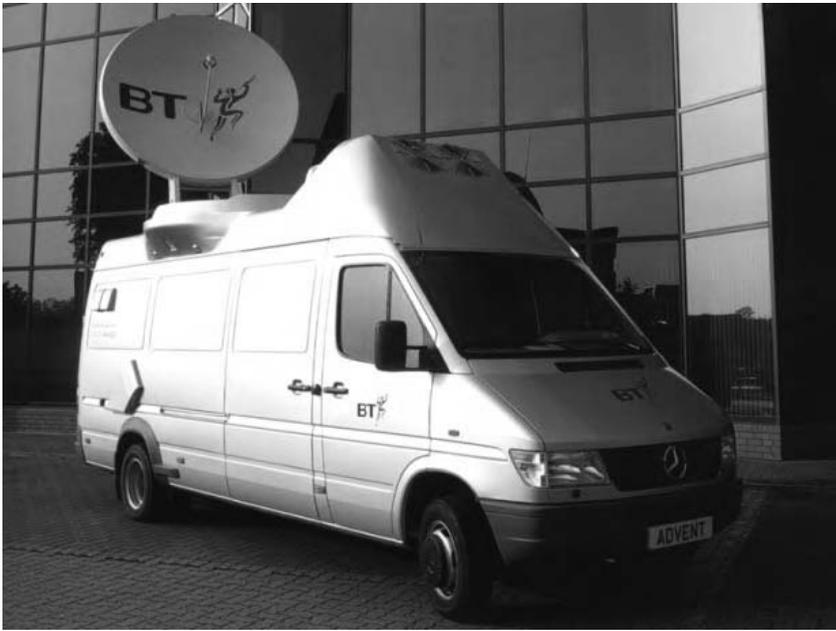
**Figure 7.26** Transportable/mobile video uplink antenna system (photo courtesy of Advent Communications).
