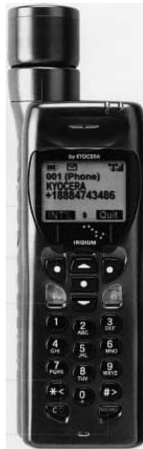
**Figure 1.9** First-generation MSS handheld mobile phone for the Iridium system (photo courtesy of Kyocera).
