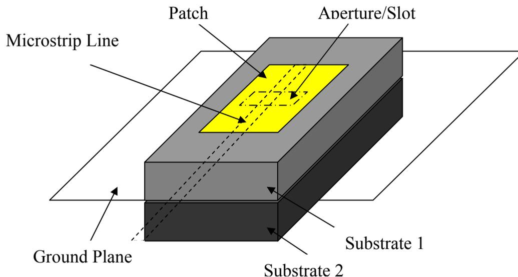
Figure 3.5 Aperture-coupled feed
