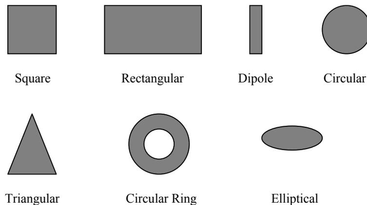
Figure 3.2 Common shapes of microstrip patch elements
