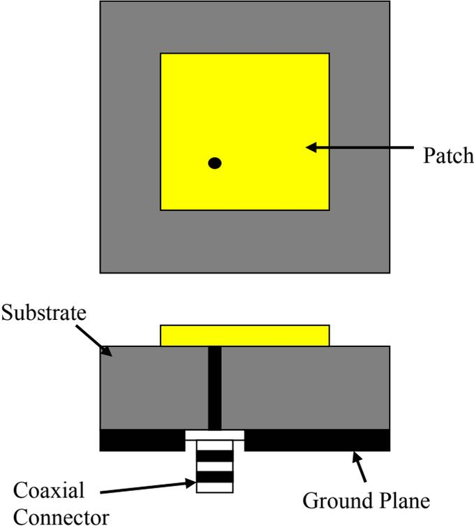
Figure 3.4 Probe fed Rectangular Microstrip Patch Antenna
