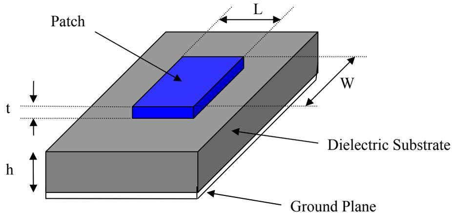
Figure 3.1 Structure of a Microstrip Patch Antenna
