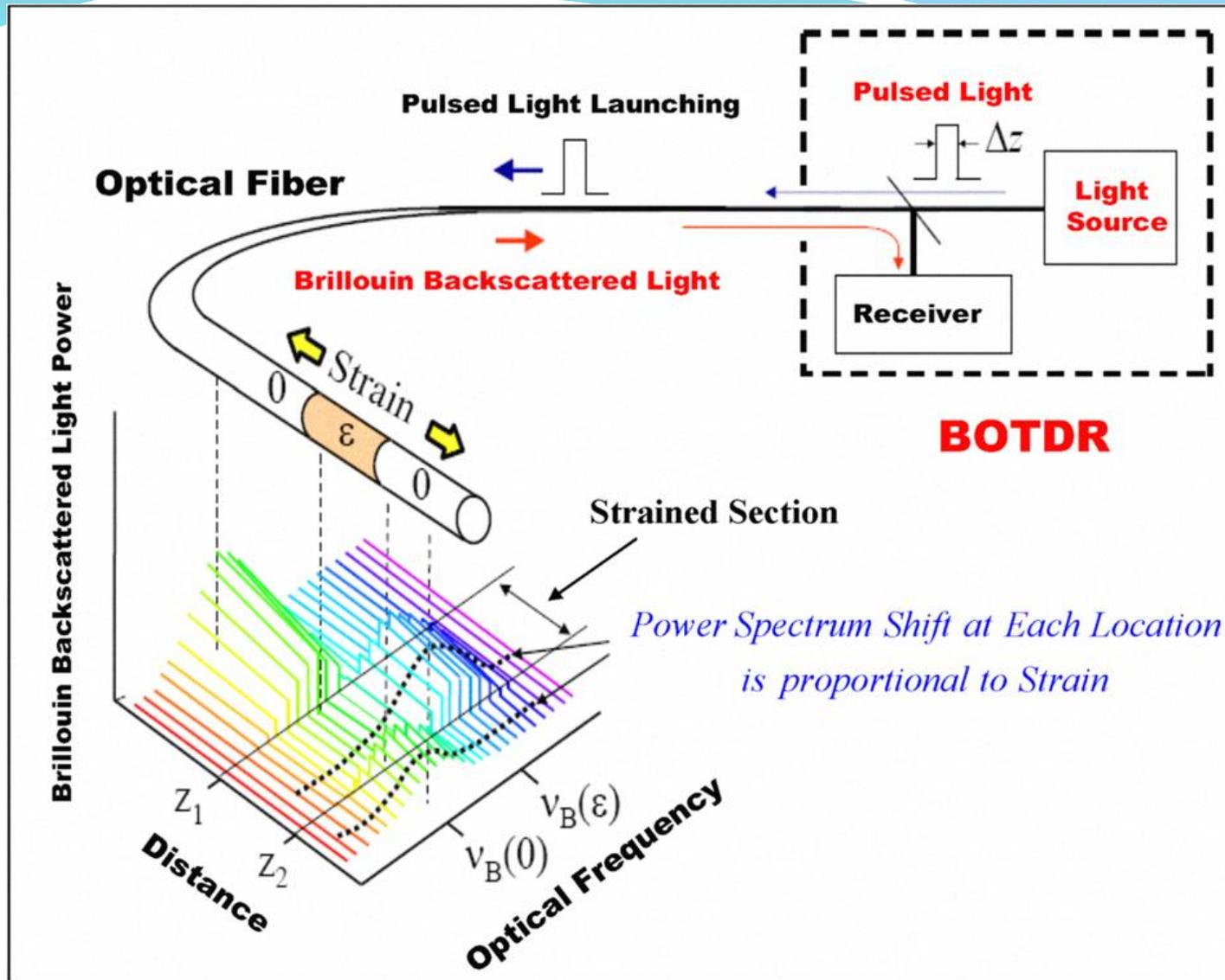
Distributed fibre optic sensing based on Brillouin scattering (adapted from Hiroshi Nasure, Mie University, Japan)
