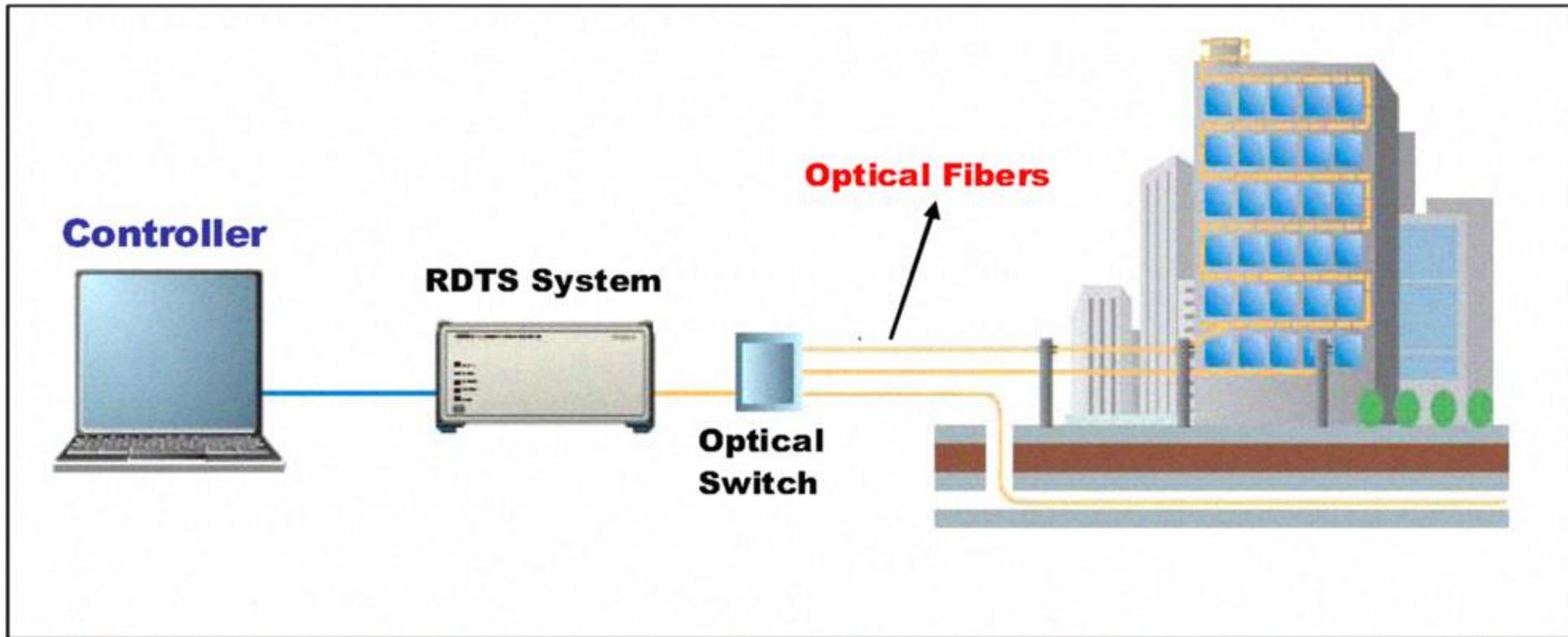
**Illustrative application of a Raman based distributed temperature measurement system in building fire detection (adapted from Yokogawa, 2007)**
