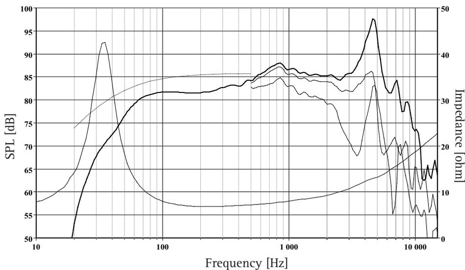
The frequency responses above show measured free field sound pressure in 0, 30, and 60 degrees angle using a 12L closed box. Input 2.83 V<sub>rms</sub>, microphone distance 0.5m, normalized to SPL 1m. The dotted line is a calculated response in infinite baffle based on the parameters given for this specific driver. The impedance is measured in free air without baffle using a 2V sine signal.
