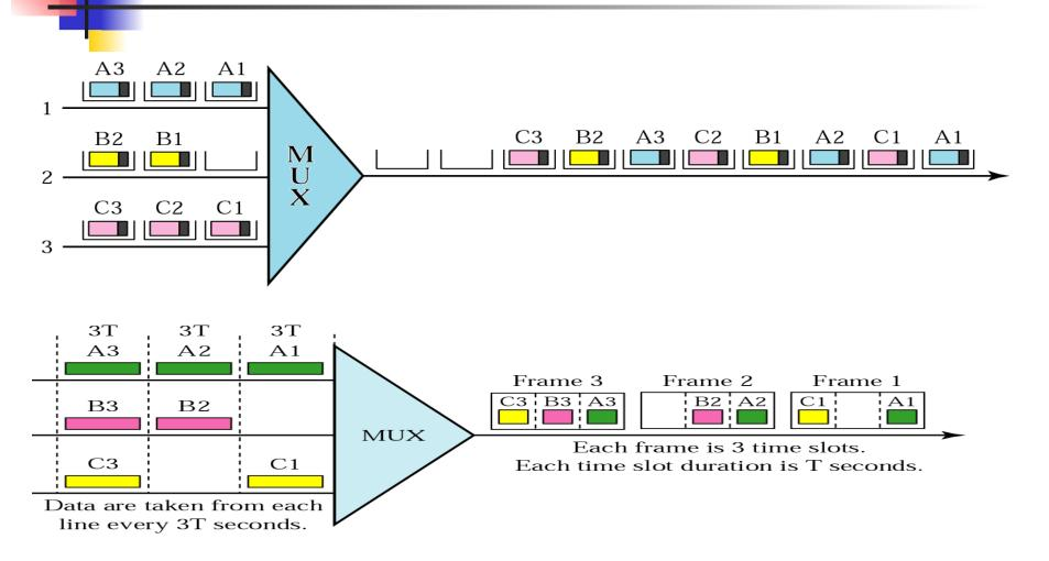
a) Asynchronous TDM : ATM multiplexers fill a slot with a cell from any input channel that has a cell.b) TDM
