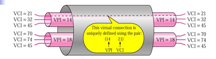
1- Transmission Path (TP): the physical connection (wire, cable, satellite, ... ) between an endpoint and a switch or between two switches.
