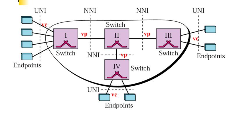
User-to-network interface (**UNI**): interface between endpoint (user access devices) and network switches. Network-to-network interface (**NNIs**): interface between switches insides the network.
