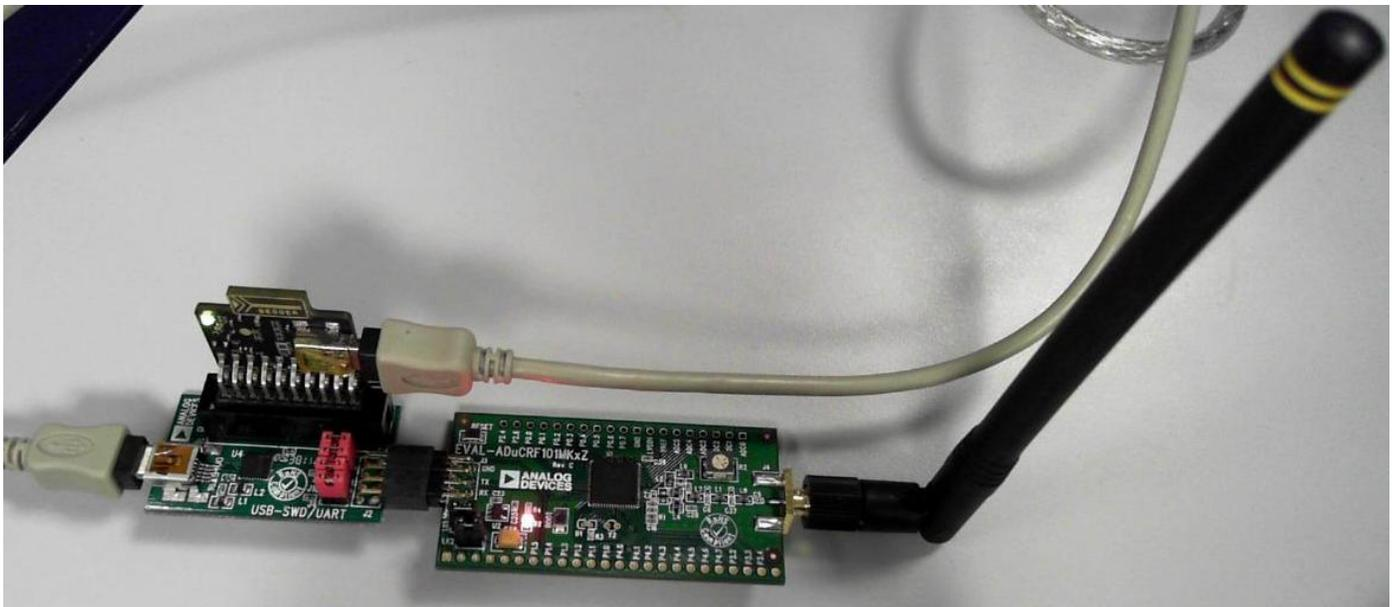
Figure 1 ADuCRF101 Mini Board and Interface Board
