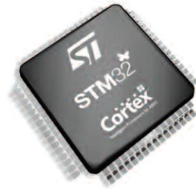
The STM32 family of 32-bit Flash microcontrollers is based on the breakthrough ARM Cortex-M3 core specifically developed for embedded applications. The STM32 family benefits from the Cortex-M3 architectural enhancements, including the Thumb-2® instruction set to deliver
