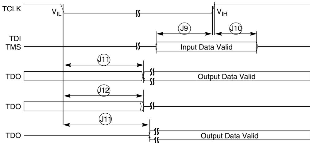
Figure 14. Test Access Port Timing
