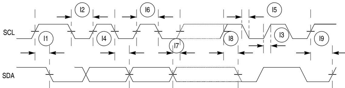
**Figure 8. I<sup>2</sup>C Input/Output Timings**
