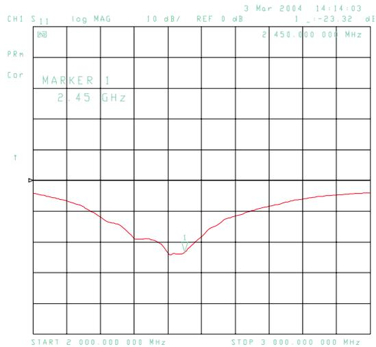
**Figure 16. F Antenna Return Loss and Bandwidth**
