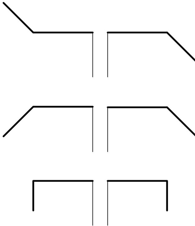
**Figure 2. Dipole Shapes to Improve Omnidirectional Characteristics**
