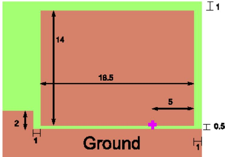
Figure 26. Patch Antenna 1
