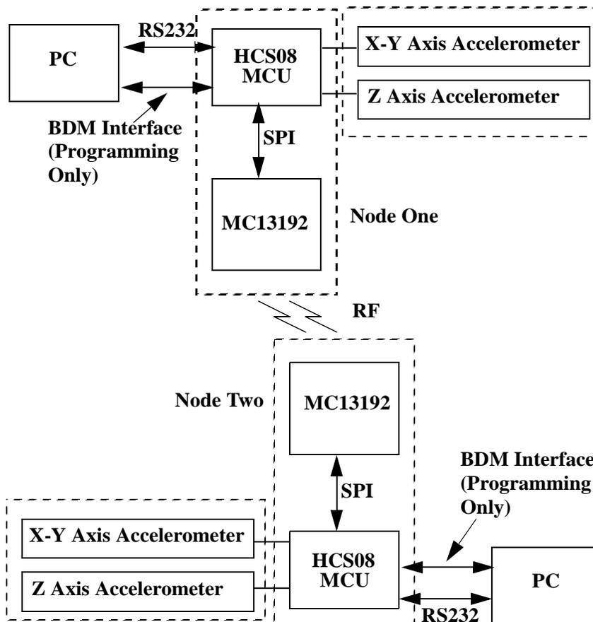
Figure 1-1. Point to Point MC13192 SARD Block Diagram
