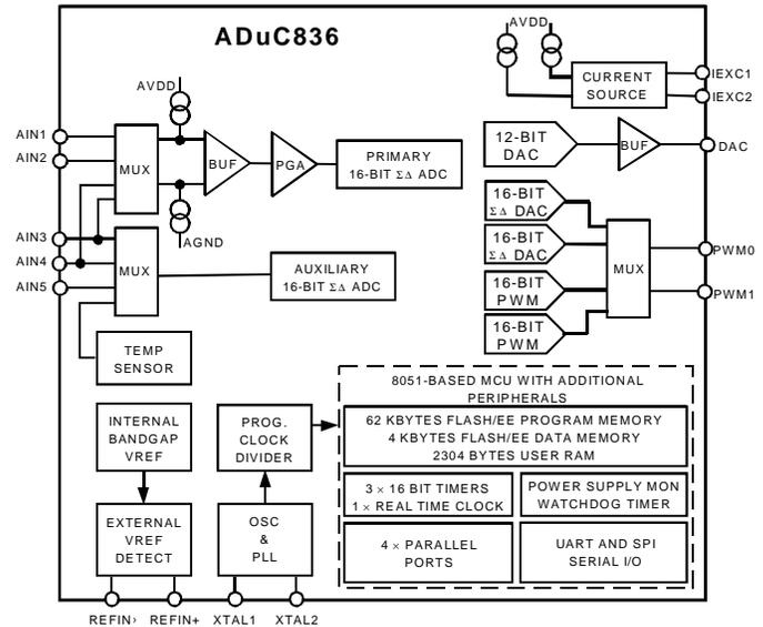
62 Kbytes of nonvolatile Flash/EE program memory are provided on-chip. 4 Kbytes of nonvolatile Flash/EE data memory, 256 bytes RAM and 2 Kbytes of extended RAM are also integrated on-chip. The program memory can be configured as data memory in datalogging applications.
