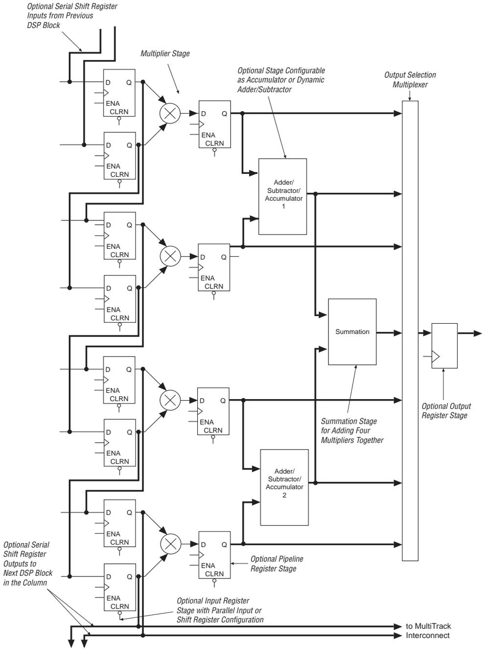
Figure 31. DSP Block Diagram for 9 × 9-Bit Configuration
