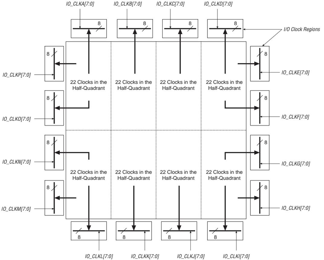
Designers can use the Quartus II software to control whether a clock input pin is either global, regional, or fast regional. The Quartus II software automatically selects the clocking resources if not specified.
