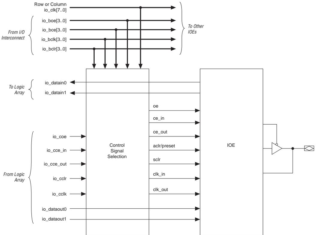
Each IOE contains its own control signal selection for the following control signals: *oe*, *ce\_in*, *ce\_out*, *aclr/preset*, *sclr/preset*, *clk\_in*, and *clk\_out*. Figure 62 illustrates the control signal selection.
