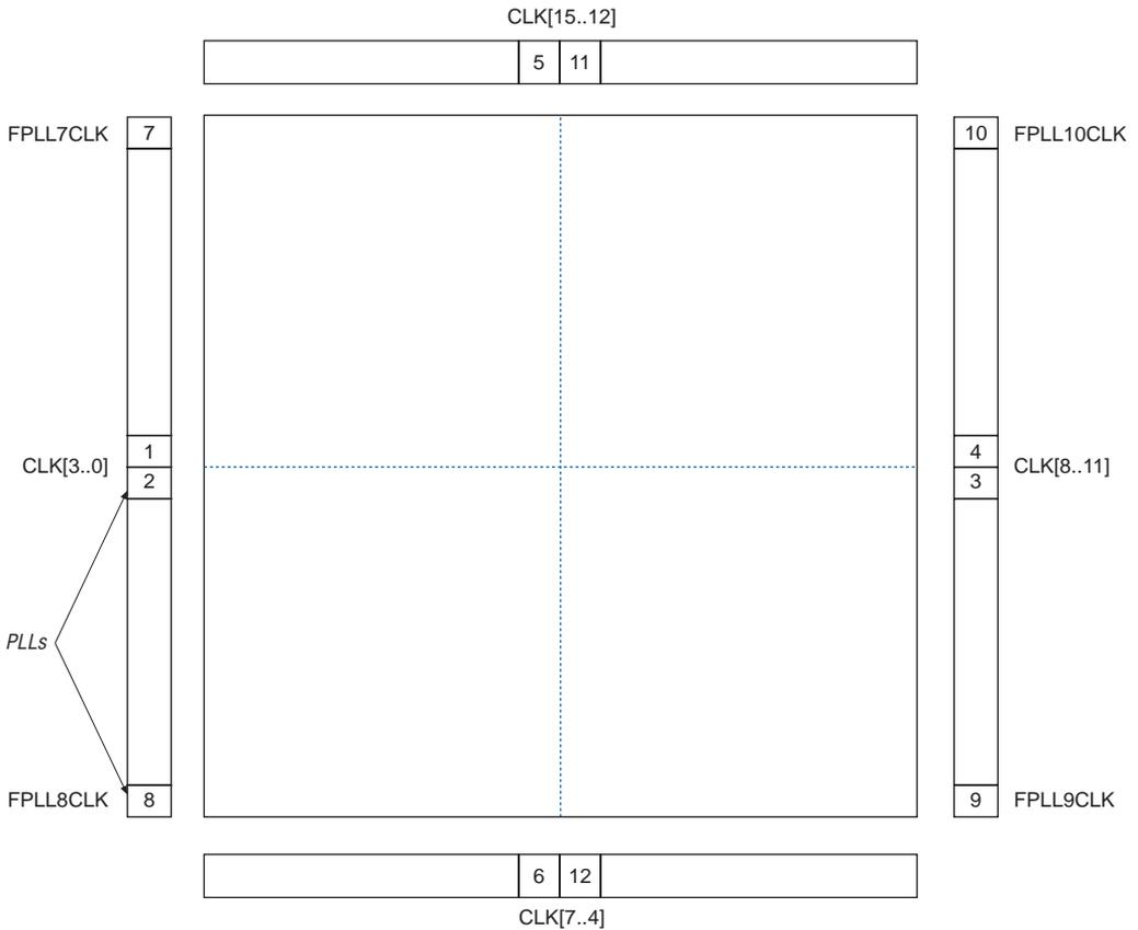
Figure 50 shows the global and regional clocking from the PLL outputs and the CLK pins.
