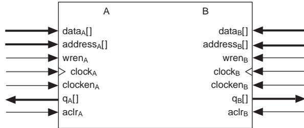
In addition to true dual-port memory, the memory blocks support simple dual-port and single-port RAM. Simple dual-port memory supports a simultaneous read and write. Single-port memory supports non-simultaneous reads and writes. Figure 13 shows these different RAM memory port configurations for TriMatrix memory.
