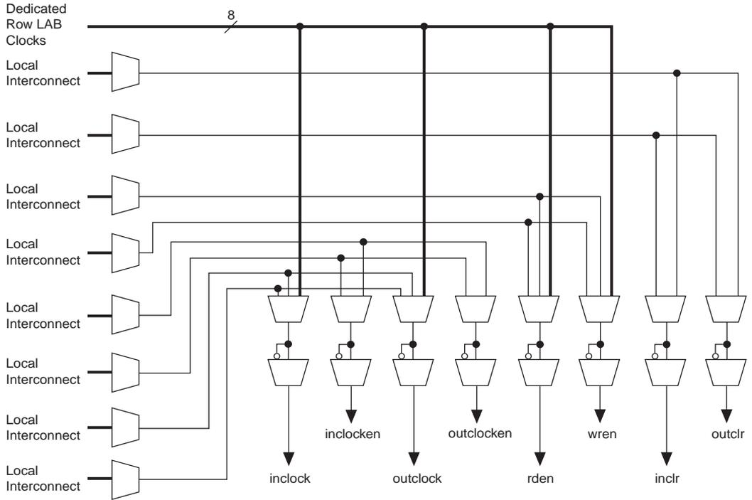
**Figure 16. M512 RAM Block LAB Row Interface**
