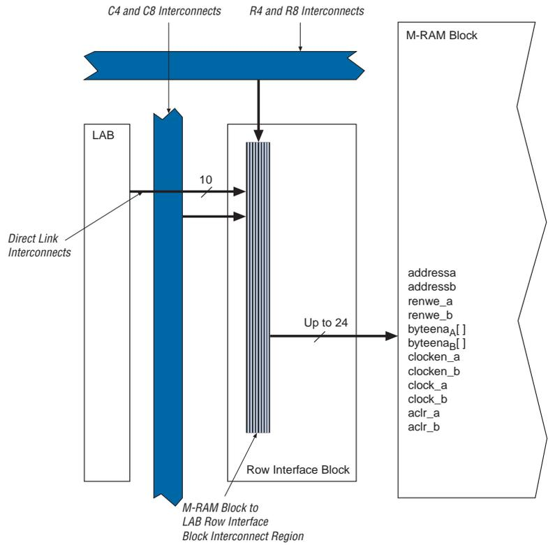
Figure 23. M-RAM Column Unit Interface to Interconnect
