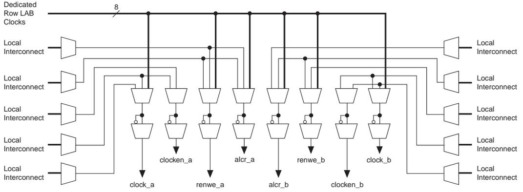
**Figure 18. M4K RAM Block LAB Row Interface**
