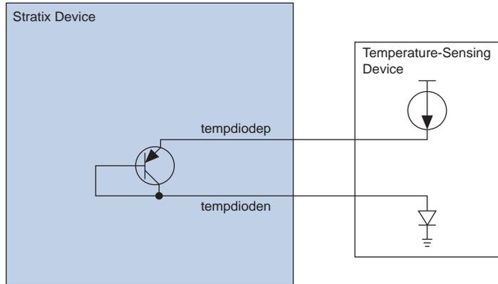
**Table 42. Temperature-Sensing Diode Electrical Characteristics**
