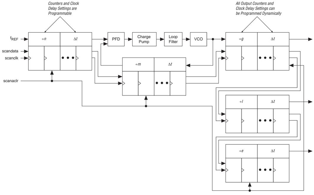
PLL reconfiguration data is shifted into serial registers from the logic array or external devices. The PLL input shift data uses a reference input shift clock. Once the last bit of the serial chain is clocked in, the register chain is synchronously loaded into the PLL configuration bits. The shift circuitry also provides an asynchronous clear for the serial registers.
