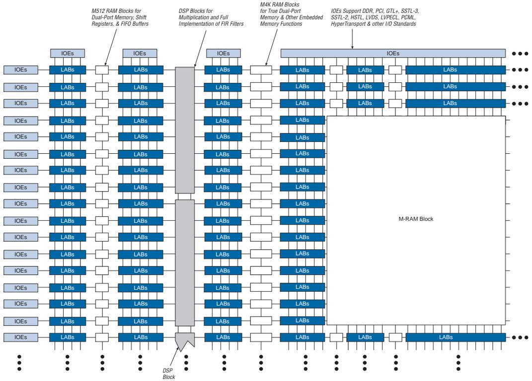
The number of M512 RAM, M4K RAM, and DSP blocks varies by device along with row and column numbers and M-RAM blocks. [Table 6](#) lists the resources available in Stratix devices.
