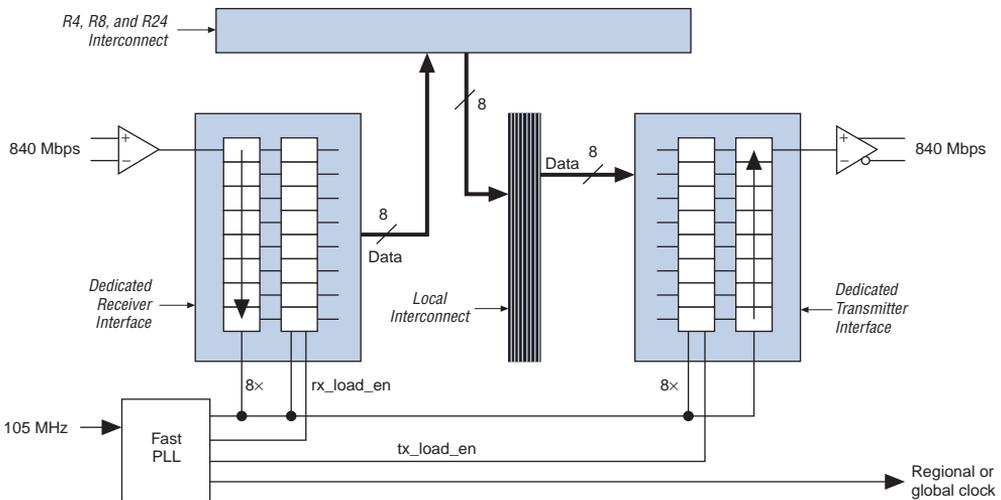
An external pin or global or regional clock can drive the fast PLLs, which can output up to three clocks: two multiplied high-speed differential I/O clocks to drive the SERDES block and/or external pin, and a low-speed clock to drive the logic array.
