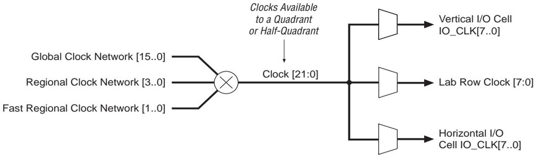
IOE clocks have horizontal and vertical block regions that are clocked by eight I/O clock signals chosen from the 22 quadrant or half-quadrant clock resources. Figures 47 and 48 show the quadrant and half-quadrant relationship to the I/O clock regions, respectively. The vertical regions (column pins) have less clock delay than the horizontal regions (row pins).
