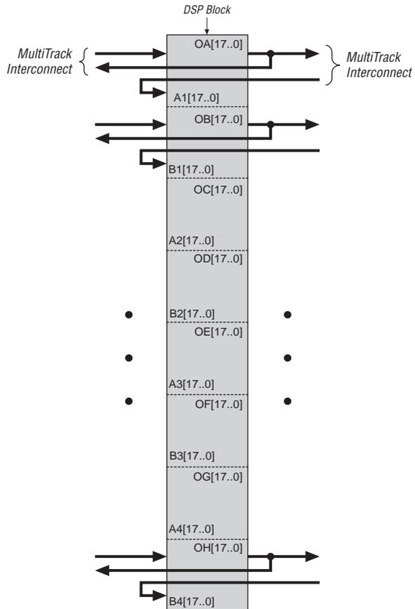
**Figure 41. DSP Block Interface to Interconnect**
