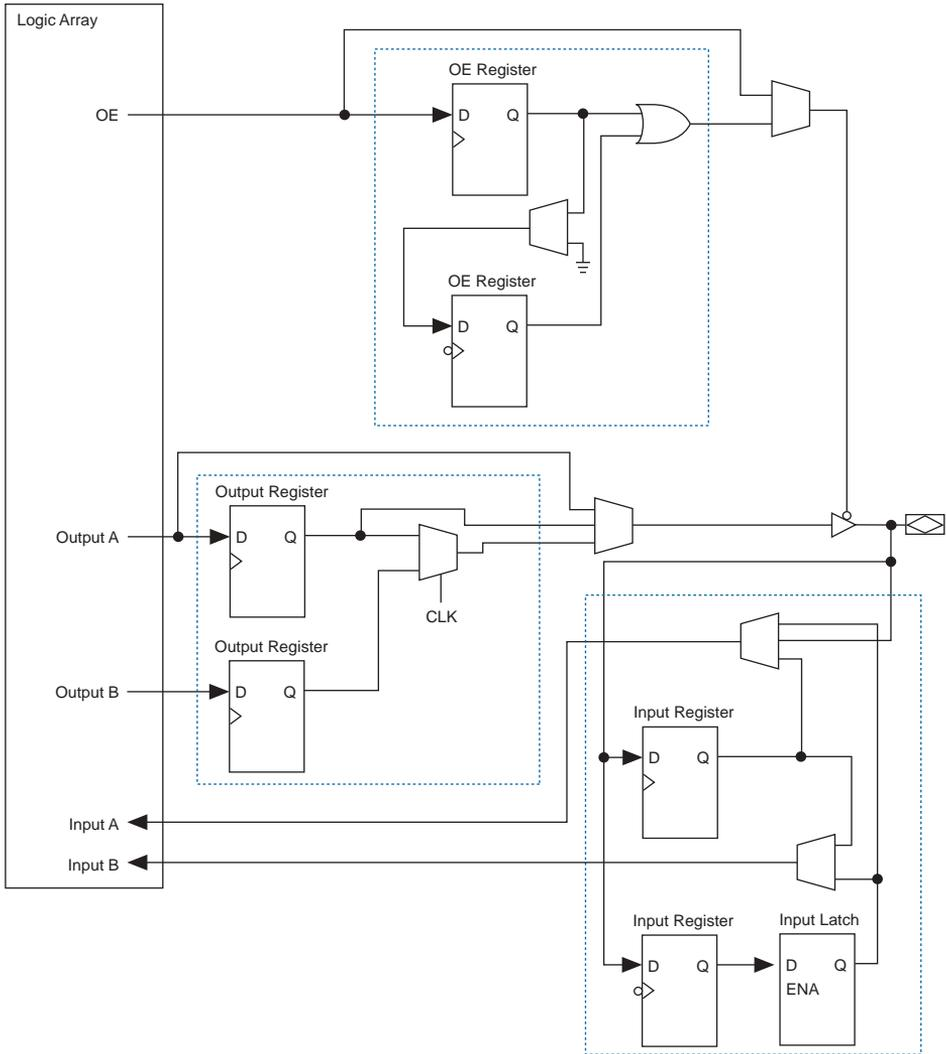
The IOEs are located in I/O blocks around the periphery of the Stratix device. There are up to four IOEs per row I/O block and six IOEs per column I/O block. The row I/O blocks drive row, column, or direct link interconnects. The column I/O blocks drive column interconnects.
