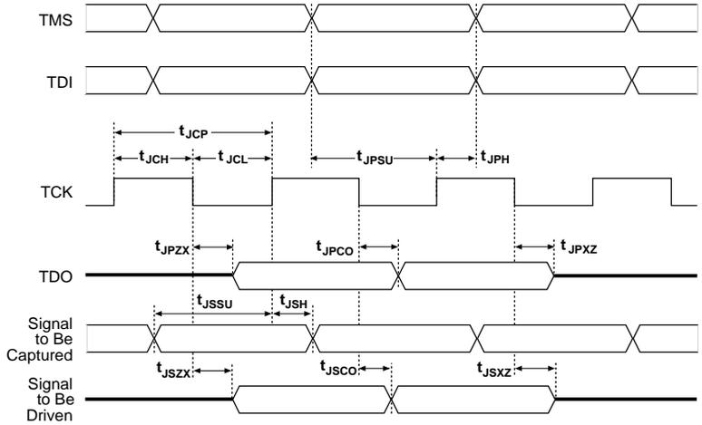
Table 40 shows the JTAG timing parameters and values for Stratix devices.
