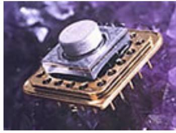
Figure 15. Shows the Silicon Sensing Sensor package with a permanent magnet mounted directly on top of the sensor element in a metal can header for sealing under vacuum.
