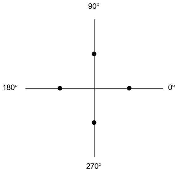
Figure 2.39 V.29 Constellation For 4800 bits/s Fallback Mode
