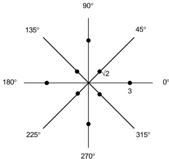
Figure 2.38 V.29 Constellation For 7200 bits/s Fallback Mode
