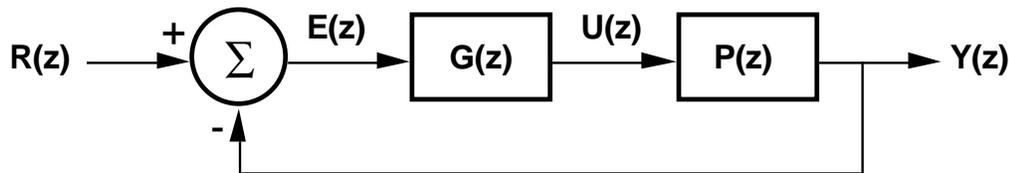
Figure 9.2 Digital Control System Model
