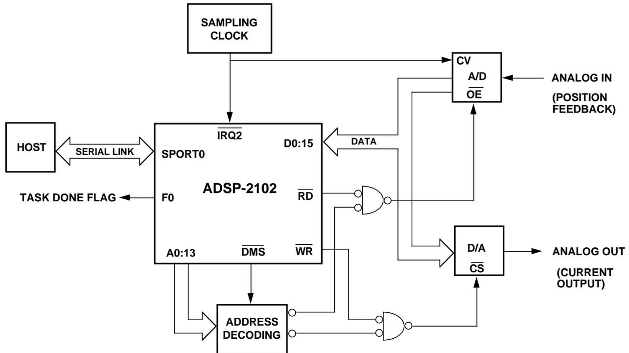
Figure 9.3 ADSP-2101-Based Actuator Controller
