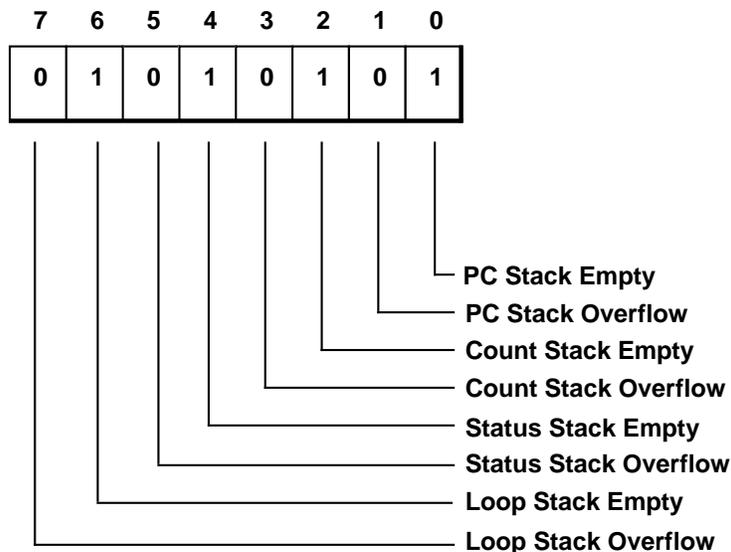
Figure 3.5 SSTAT Register (Read-Only)
