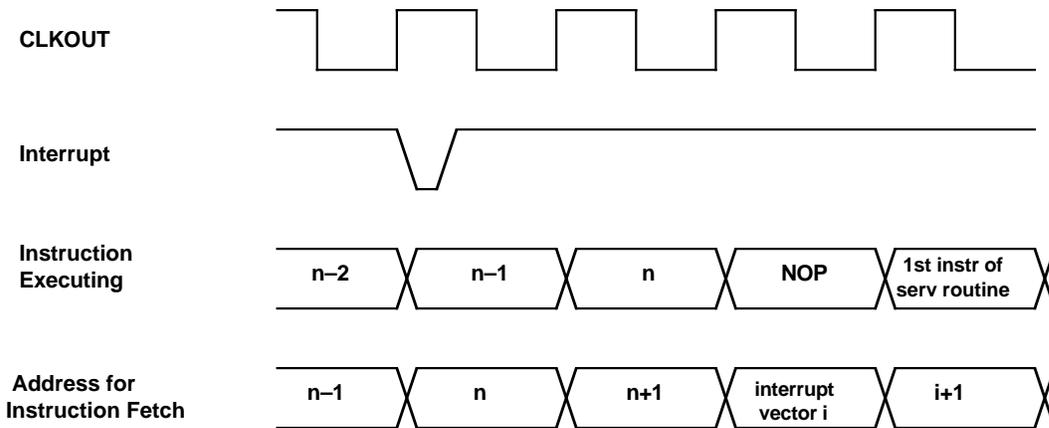
**Figure 3.2 Interrupt Latency (Timer,  $\overline{IRQx}$ , SPORT, HIP, & Analog Interrupts)**
