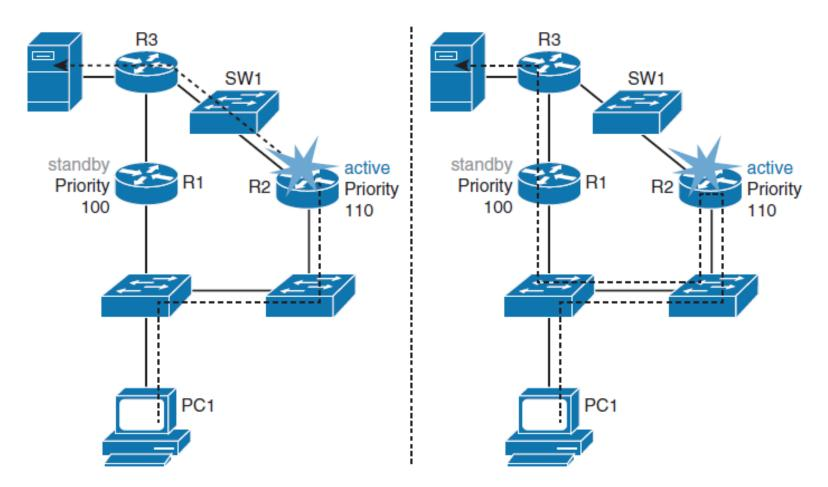
HSRP has a built-in mechanism for detecting link failures and starting the HSRP reelection process.
